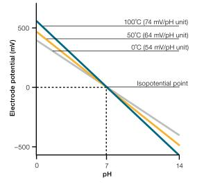
Figure 1. Change in Nerstian slope of an electrode with temperature.
