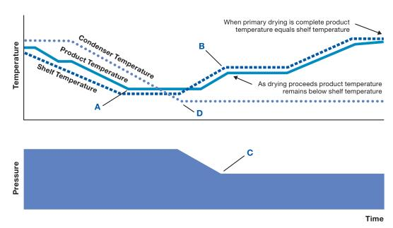
Figure 4: Typical Sublimation Cycle found in system utilizing Tray Dryer with shelves.
