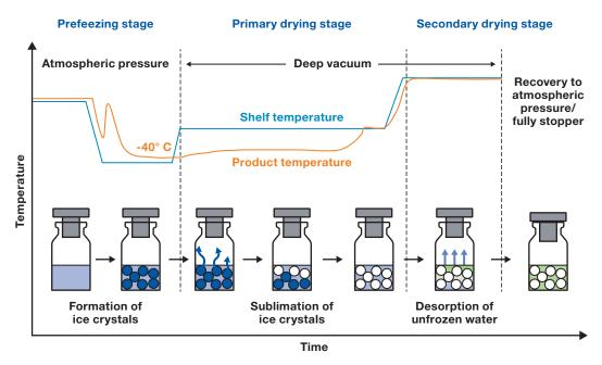
Figure 1: Stages of Freeze Drying
