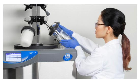
In the manifold method, flasks are individually attached to the ports of a drying chamber.
