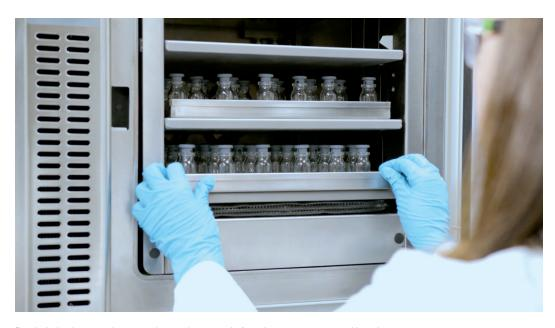
Batch drying in a tray dryer permits precise control of product temperature and heat input.
