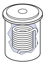
**Figure 3:** Collecting system acts as a cold trap to collect moisture leaving the frozen product.
